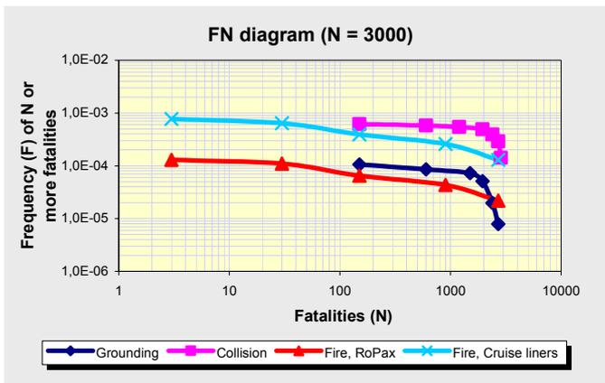
Fig. 6. FN diagram for ships with 3000 people on board.
