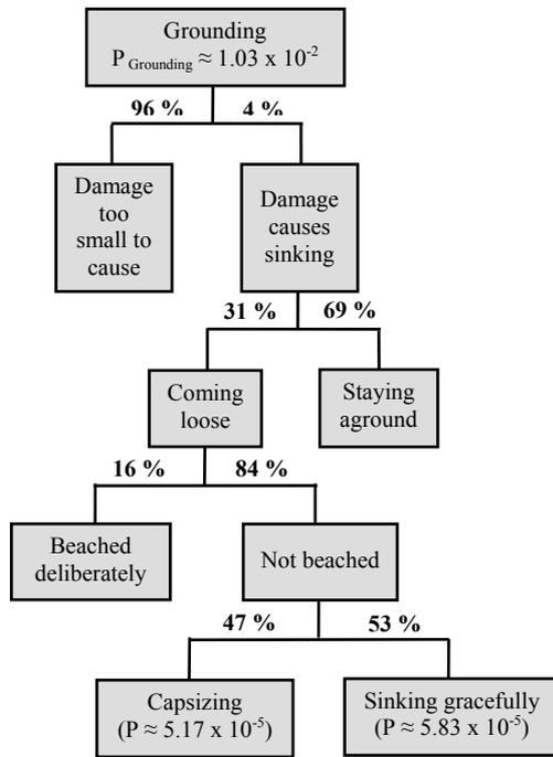
Fig. 4. Model for grounding of passenger ships
