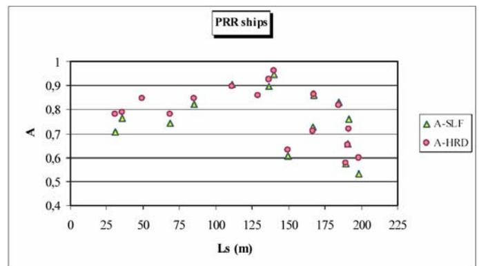
Fig. 2. Attained subdivision index  $A$  for passenger ro-ro ships as a function of the total ship length, as calculated by the HARDER project
