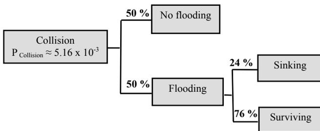
Fig. 1. Event tree for collision of passenger ships
