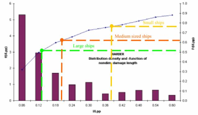
Fig. 5. Grounding damages distribution function from the HARDER project
